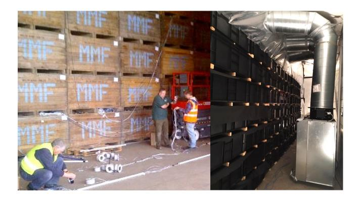
Much of the project has involved working in commercial stores to benchmark current performance; this has been produced using empirical data gathered from commercial stores (above, left) but also measurements taken from a 30% scale store (above, right) constructed at SBCSR and used to assess the impact of changes to the air system and box layout.
